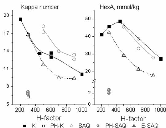
Figure 1: Kappa number and HexA content *versus* the H-factor for modified alkaline pulping
