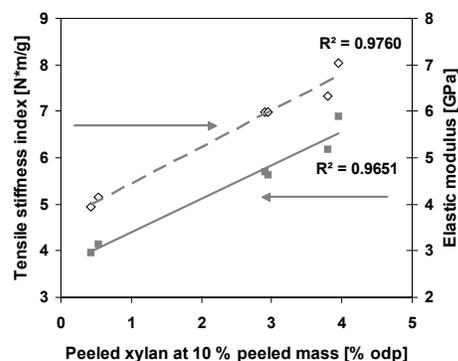
Figure 4: Tensile stiffness index and elastic modulus beaten at 4500 revolutions in the PFI mill as a function of surface xylan of unbleached eucalypt pulps
