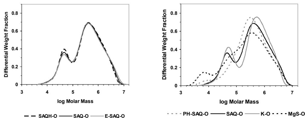
Figure 5: Molecular mass distribution of SAQ, E-SAQ, SAQH pulps and PH-SAQ, SAQ, K and MgS pulps after oxygen delignification
